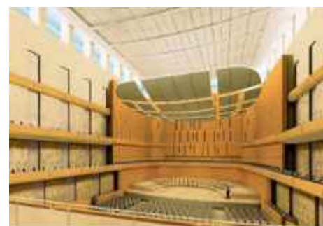
Figure 2.08 Suspended ceiling for acoustic purposes
