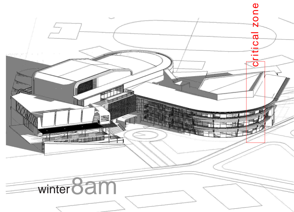
Figures 6.02 to 6.03. Critical zones as determined by perpendicular angle of incidence of sunlight during early hours of day. Occupation does not occur till 9 am.
