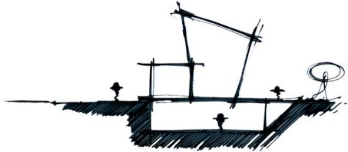
Figure 122: Typical Section C - Build Structure Half in the Ground and build the balance on Ground level.
