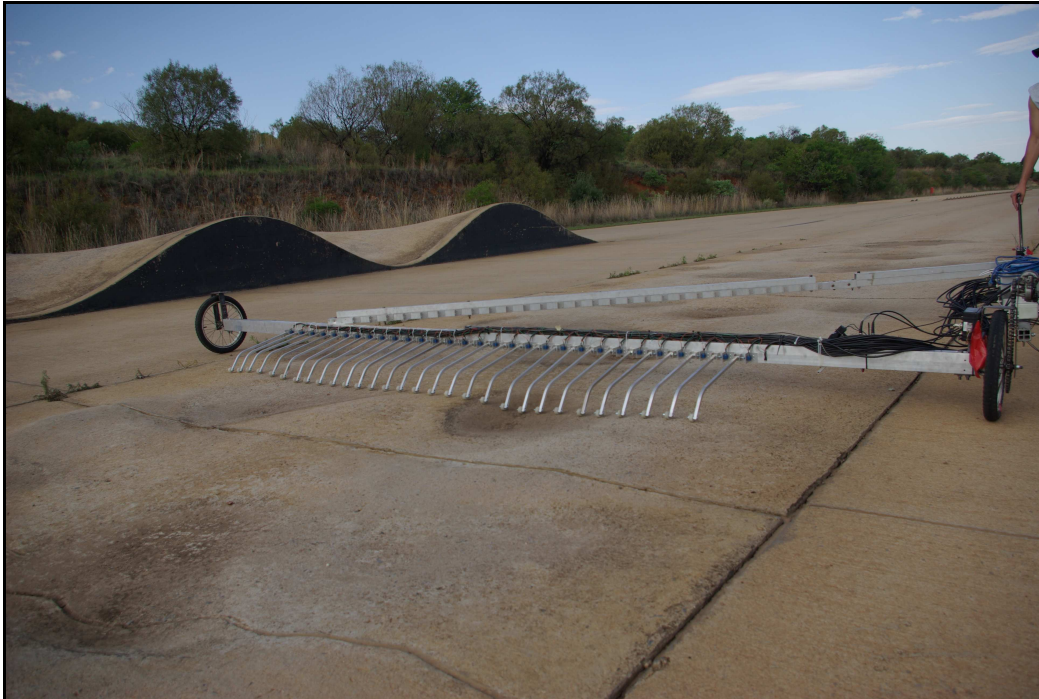
Figure 78: The Can-Can Machine profiling the Fatigue track.
