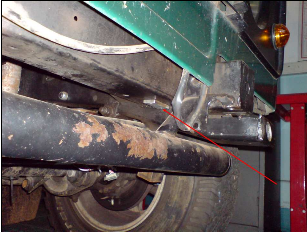
Figure 104: Placement of front accelerometer on chassis of Land Rover Defender 110.
