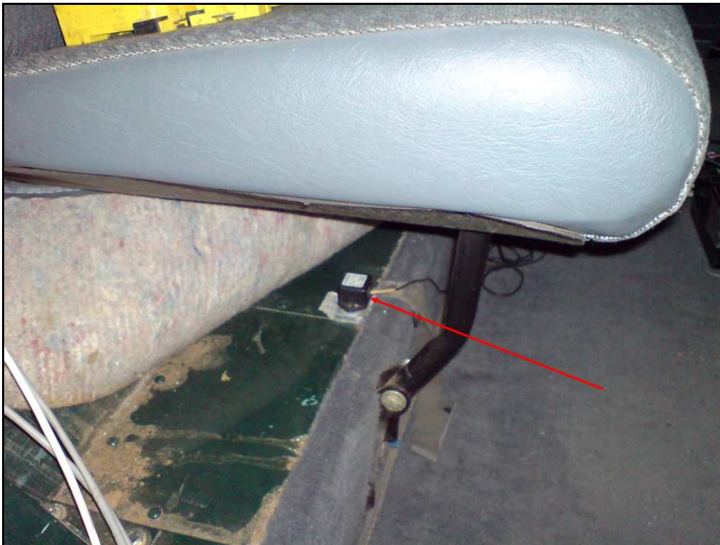
Figure 103: Placement of rear accelerometers in Land Rover Defender 110.
