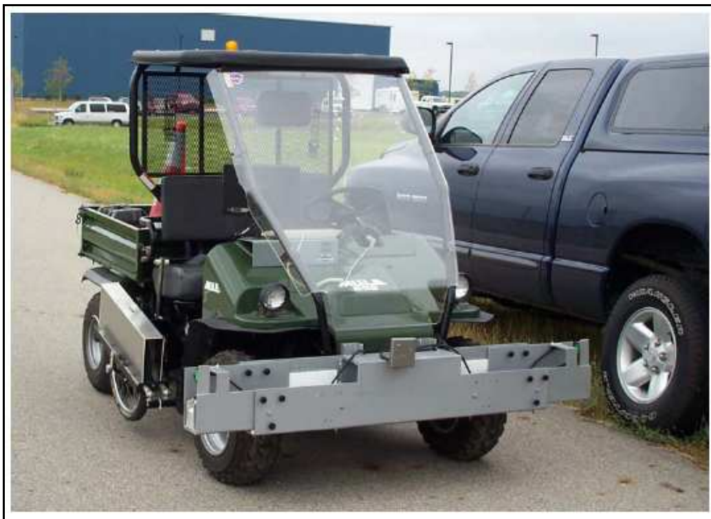
Figure 5: International Cybernetics Corporation Lightweight Profilometer, profiling moderately rough asphalt (Karamihas and Gillespie, 2002).
