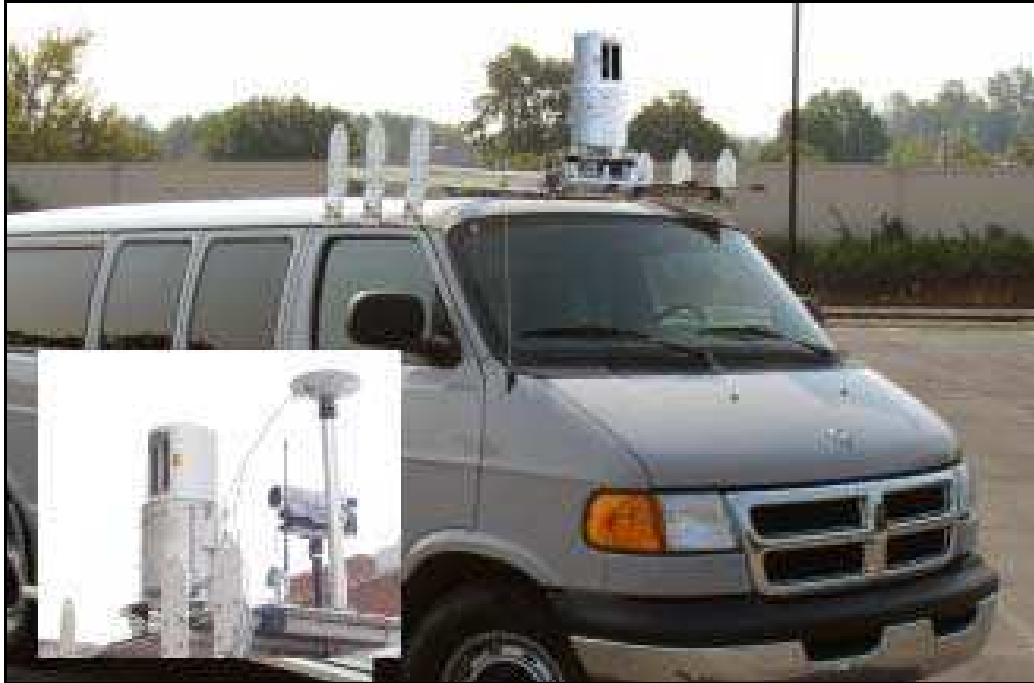
Figure 16: UTK's Mobile Scanning System consisting of a vehicle, laser range scanner, GPS, INS and high-resolution video camera (Grinstead et.al., 2005).
