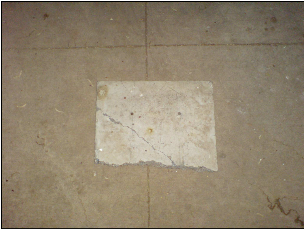
Figure 54: Test block for Laser Scanner with 500 x 360 x 58 mm concrete block on a flat surface.
