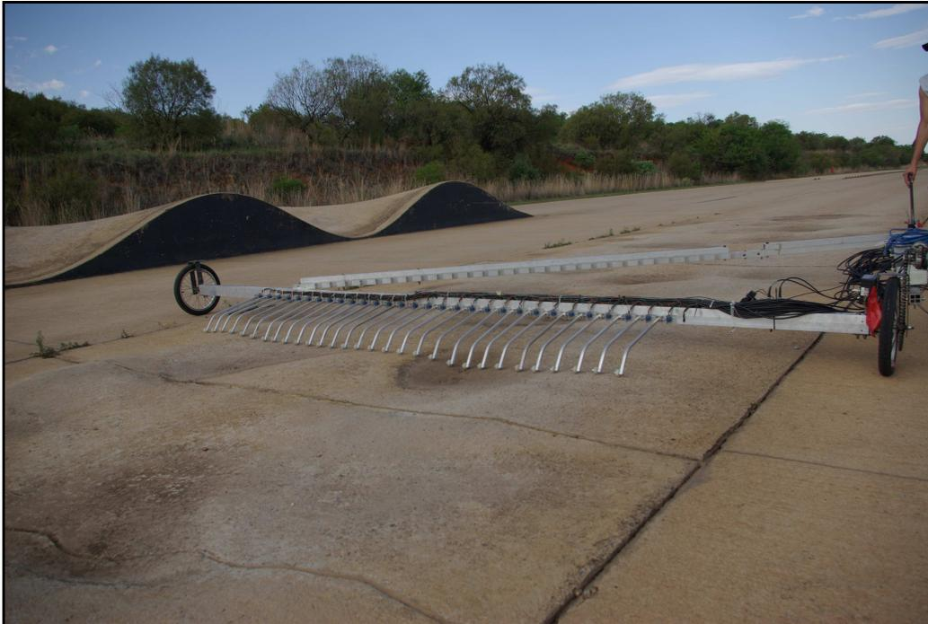
Figure 78: The Can-Can Machine profiling the Fatigue track.
