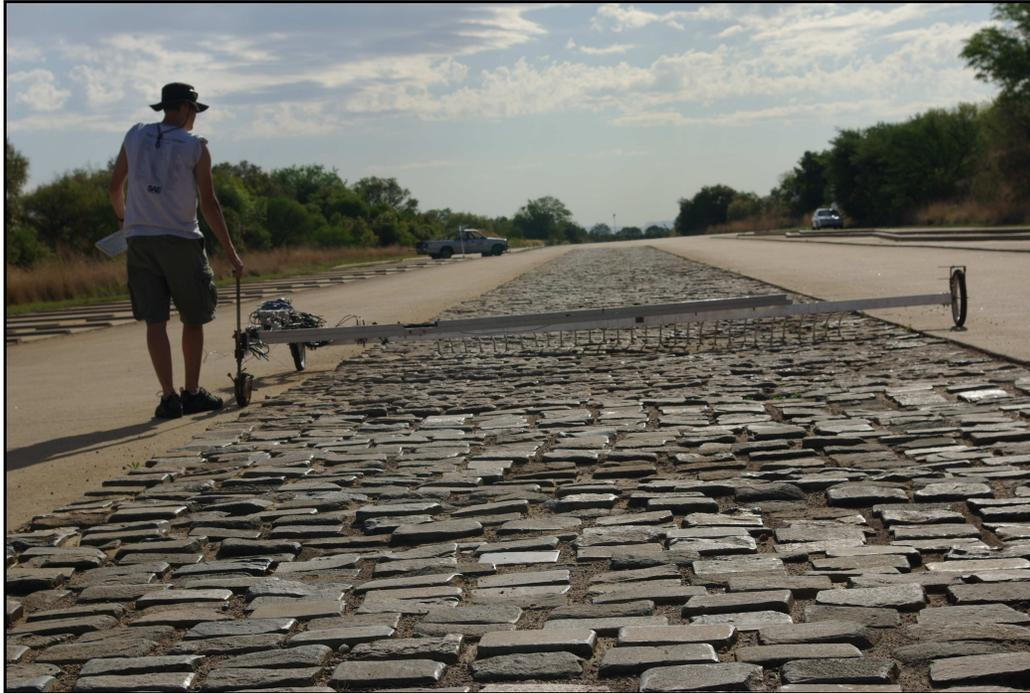
Figure 68: Can-Can Machine profiling Belgian paving.
