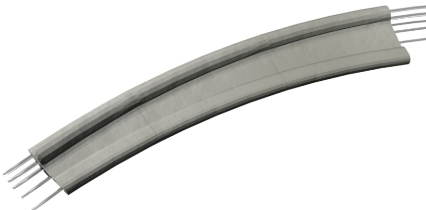
Three vault segments pulled together with cables Fig.95
