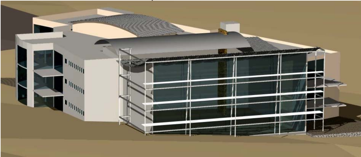
Fig. 103 - Three dimensional view of north façade and louver panel – design development phase 2.
