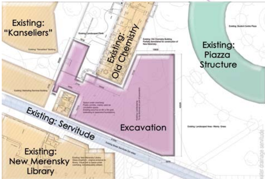
Figure 6.1: Plan: Site Excavation
