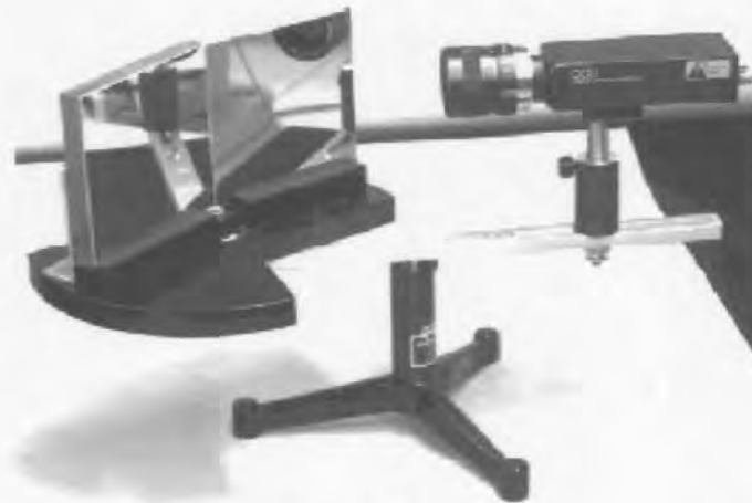
Figure 2.10 Catadioptric Stereo Sensor (Picture from [Gluckman & Nayar])
