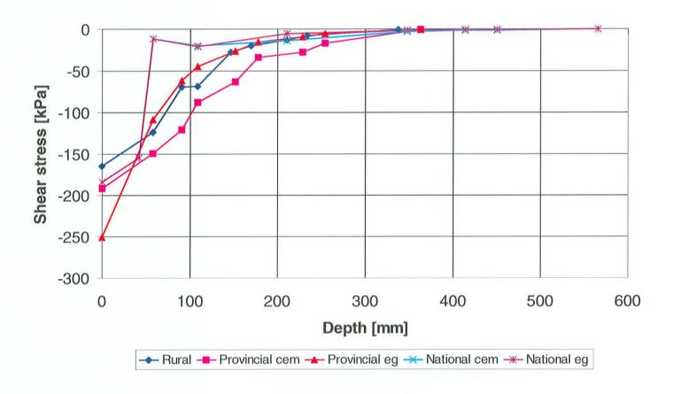
Figure 6.16: Typical shear stresses (50<sup>th</sup> percentile load) as calculated using the MCL method.
