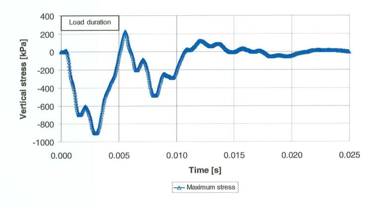
Figure 6.12: Typical vertical stresses (95<sup>th</sup> percentile load) as calculated using MCL method for rural pavement structure.
