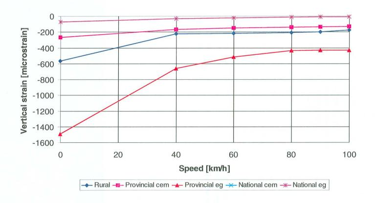
Figure 6.22: Typical vertical strain (50<sup>th</sup> percentile load) against speed as calculated using MCL method.
