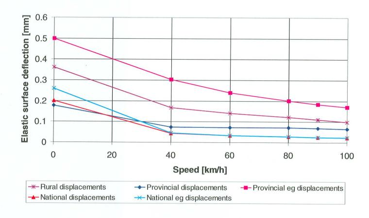
Figure 6.8: Typical elastic surface deflections (50<sup>th</sup> percentile loads) as calculated using MCL method.
