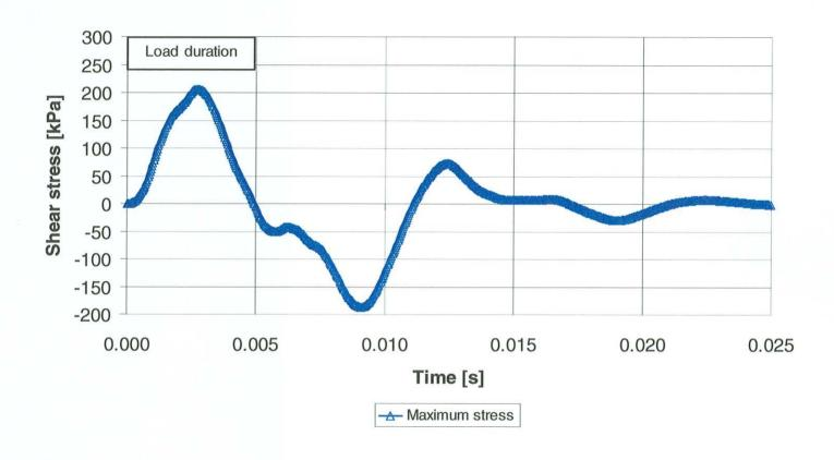
Figure 6.18: Typical shear stresses (95<sup>th</sup> percentile load) as calculated using the MCL method.
