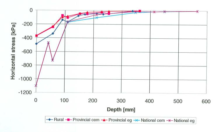
Figure 6.13: Typical horizontal stresses (50<sup>th</sup> percentile load) as calculated using the MCL method.
