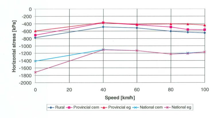
Figure 6.14: Typical horizontal stresses (50<sup>th</sup> percentile load) against speed as calculated using the MCL method.
