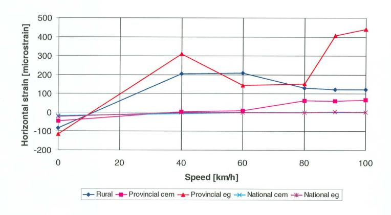
Figure 6.20: Typical horizontal strain (50<sup>th</sup> percentile load) against speed as calculated using the MCL method.
