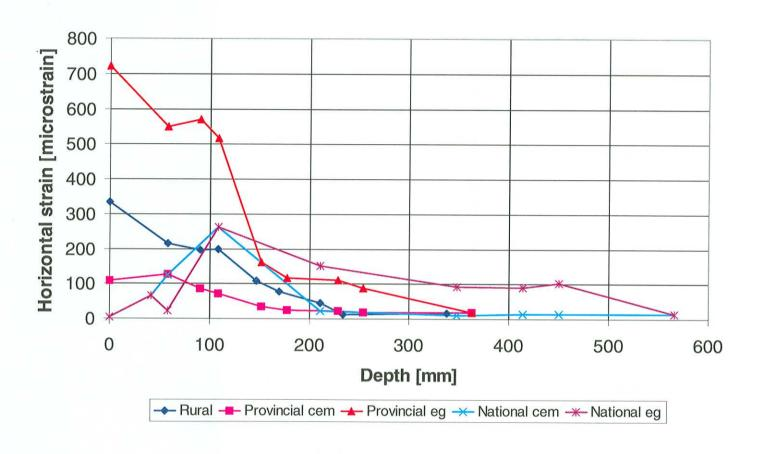
Figure 6.19: Typical horizontal tensile strain (50<sup>th</sup> percentile load) as calculated using the MCL method.
