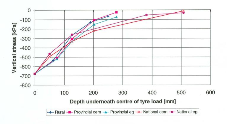
Figure 6.4: Typical vertical stress data (under centre of load) for pavements evaluated using 50<sup>th</sup> percentile static load.
