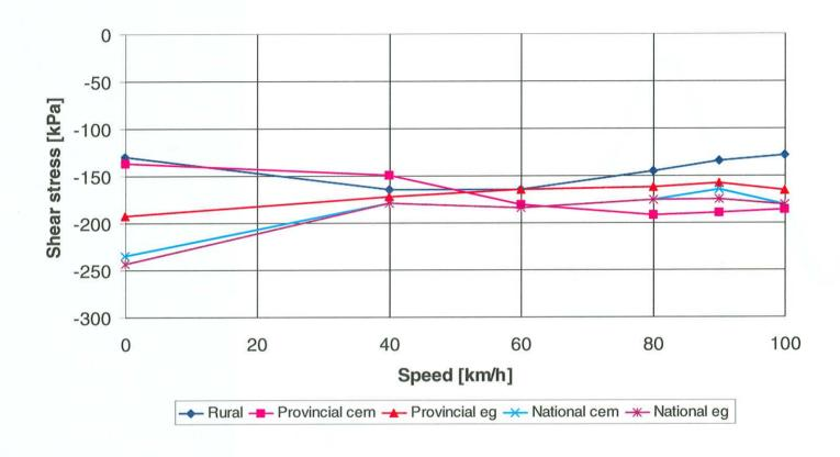
Figure 6.17: Typical shear stresses (50<sup>th</sup> percentile load) against speed as calculated using the MCL method.
