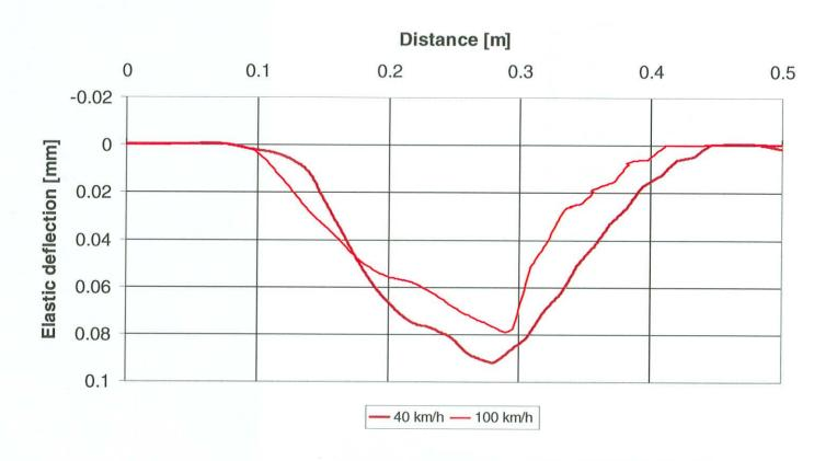
Figure 6.9: Typical elastic surface deflection bowls (90<sup>th</sup> percentile loads) on provincial cemented pavement) as calculated using MCL method.
