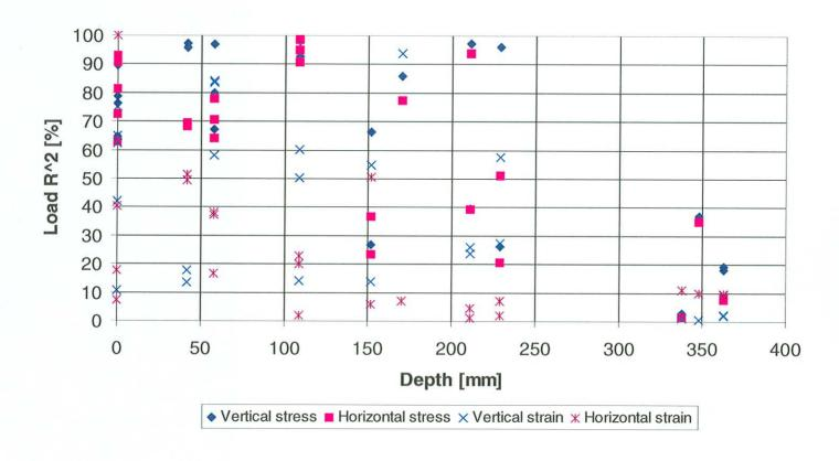
Figure 6.23: Correlations obtained through statistical analysis of applied load magnitudes and calculated stresses.
