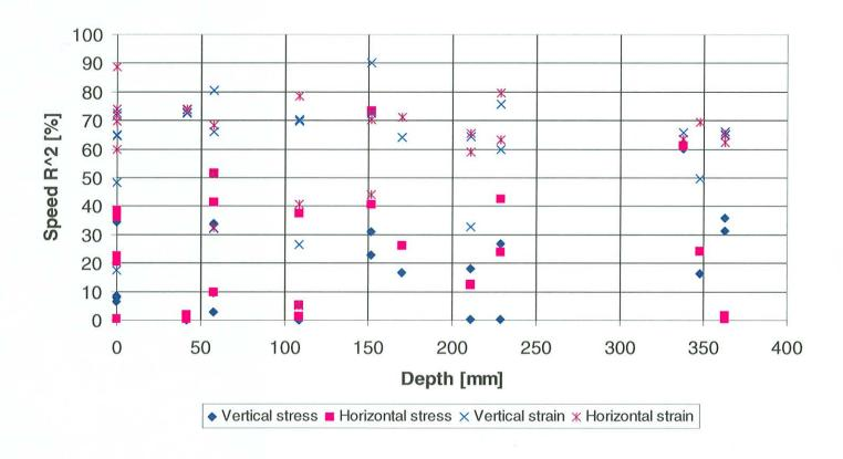
Figure 6.24: Correlations obtained through statistical analysis of applied speed and calculated stresses.
