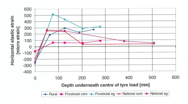
Figure 6.3: Typical horizontal tensile strain data (under centre of load) for pavements evaluated using 50<sup>th</sup> percentile static load.
