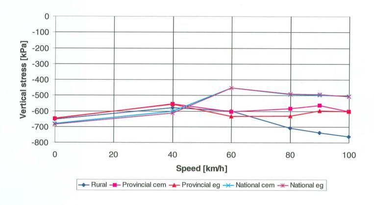
Figure 6.11: Typical vertical stresses against speed (50<sup>th</sup> percentile load) as calculated using MCL method.
