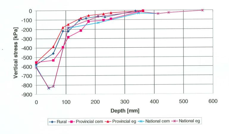
Figure 6.10: Typical vertical stresses (50<sup>th</sup> percentile load) as calculated using MCL method.
