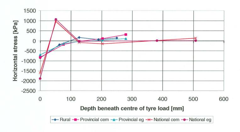
Figure 6.5: Typical horizontal stress data (under centre of load) for pavements evaluated using 50<sup>th</sup> percentile static load.
