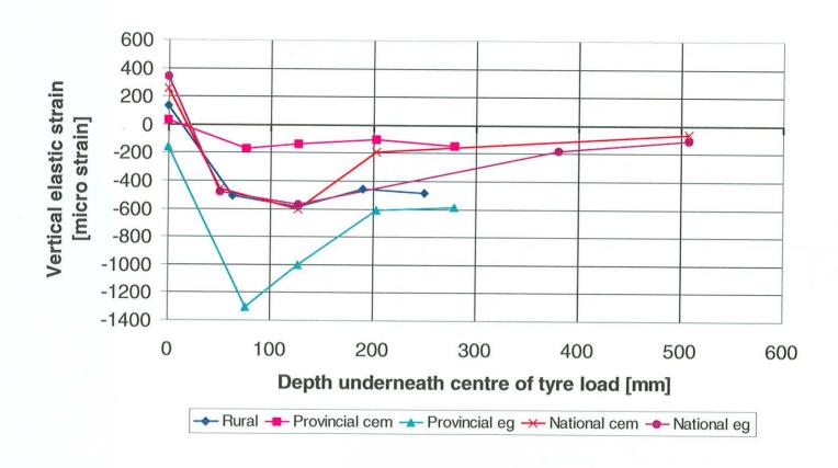
Figure 6.2: Typical vertical strain data (under centre of load) for pavements evaluated using 50<sup>th</sup> percentile static load.
