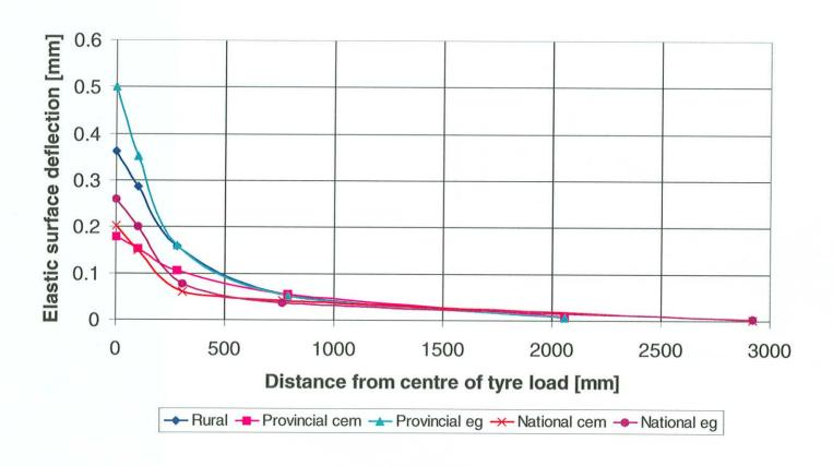
Figure 6.1: Typical elastic surface deflection data (under centre of load) for pavements evaluated using 50<sup>th</sup> percentile static load.
