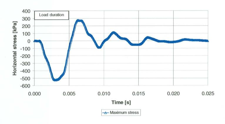
Figure 6.15: Typical horizontal stresses (95<sup>th</sup> percentile load) as calculated using the MCL method for a rural pavement structure.
