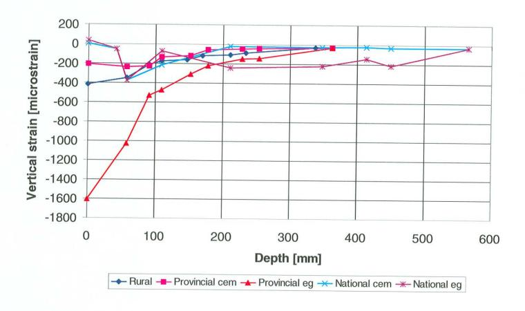
Figure 6.21: Typical vertical compressive strain (50<sup>th</sup> percentile load) as calculated using the MCL method.
