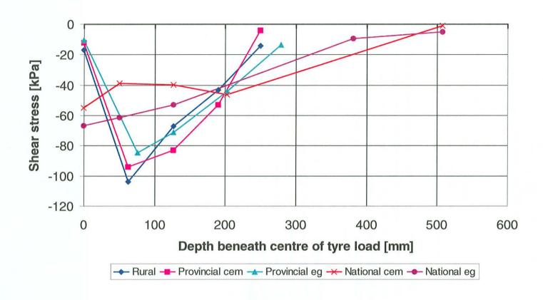
Figure 6.6: Typical shear stress data (under edge of load) for pavements evaluated using 50<sup>th</sup> percentile static load.
