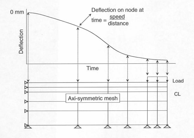
Figure 6.7: Graphical explanation of development of deflection bowls from axi-symmetric finite element data using superposition method.
