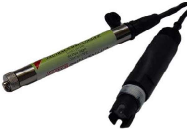
Figure 1. TruTrack Data Logger and pH-HR probe used for the assembly of a submersible pH measuring device
