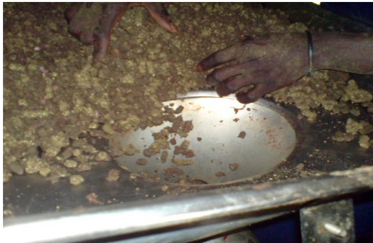
Plate 20: Once the two diets have been thoroughly mixed, the new mixture is passed into the mincer to form the new treatment diet
