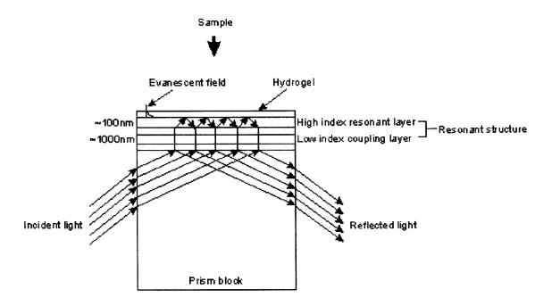
Figure 4.1: Configuration of the resonant mirror sensor device. Only one angle of incident light is shown for clarity. (Adapted from IAsys Plus User's Guide, 2000).
