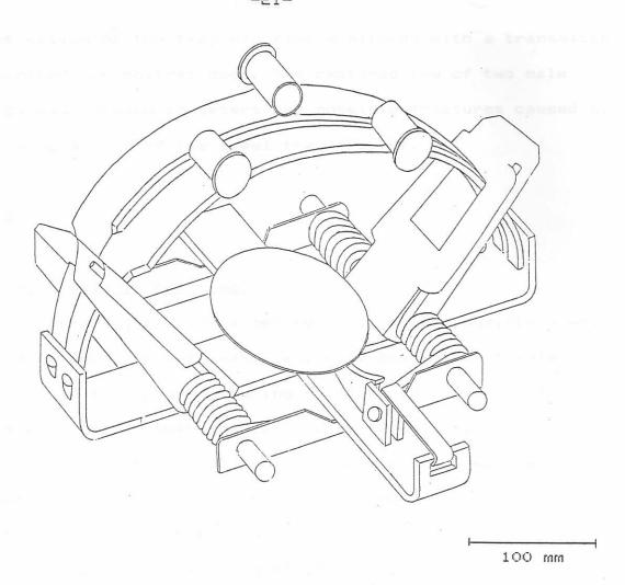
Figure 6 : The Horizontal Dubble Coil Spring Steel Trap.
