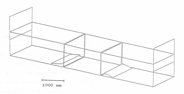
Figure 4 : The Boon Double Door Walk-in Box Trap.
