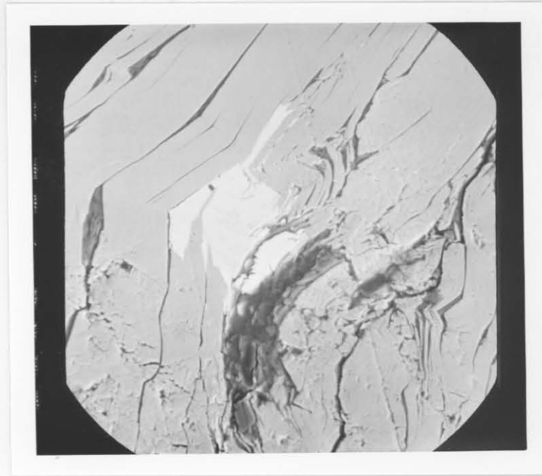
Fig. 4.13.: Kinkbands of molybdenite are characteristic. Bismuth-telluride occurs in the molybdenite ore. 20 kV. 390x. VW-1. Varschwater 23JS.
