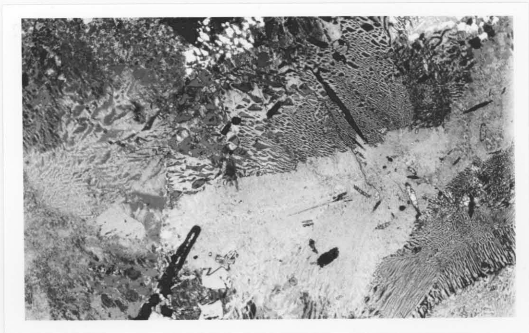
Fig. 3.13.: Laths of clinopyroxene in granophyre. The large extinction angle of 45^\circ can be seen from the position of one clinopyroxene lath. GR-43. X-Nicols. 25x. Tussenin 21JS.
