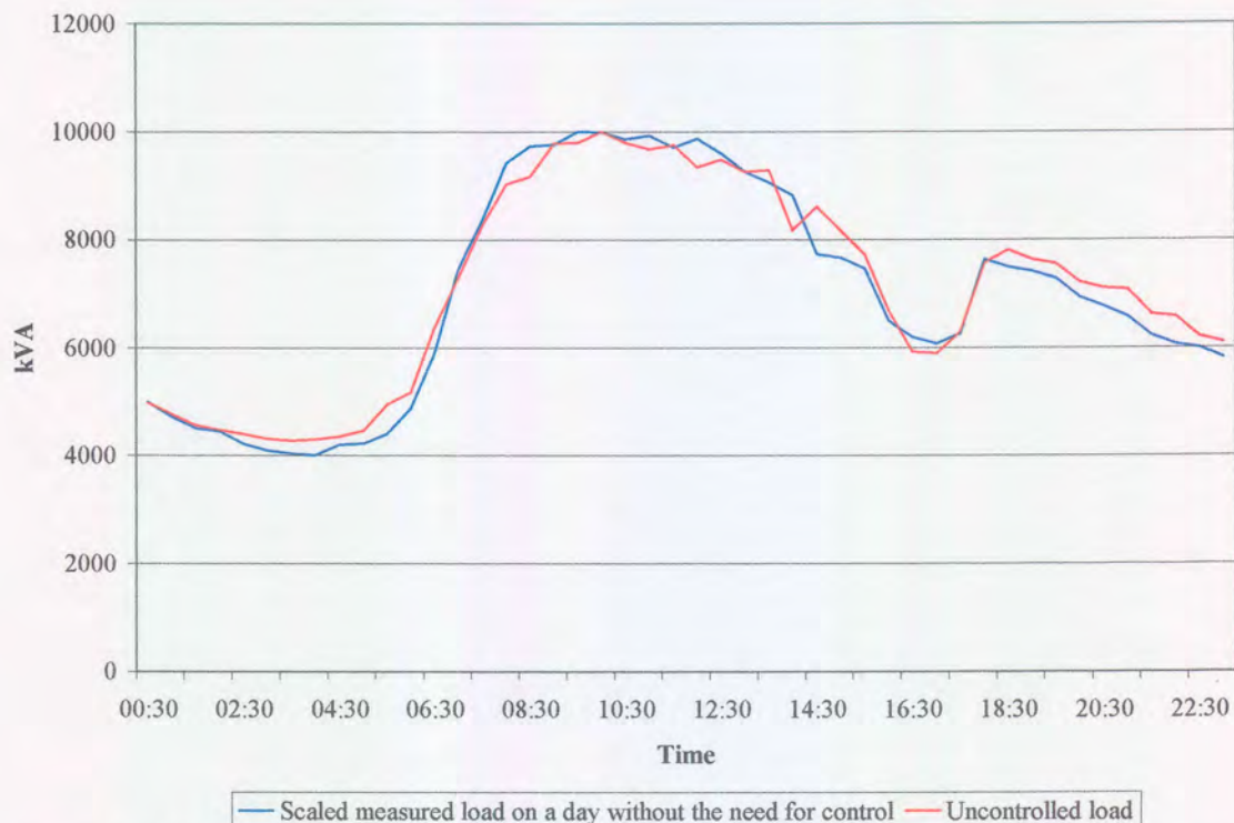
Figure 4.2. This figure shows a scaled measured load on a day without control against a day's constructed uncontrolled load.
