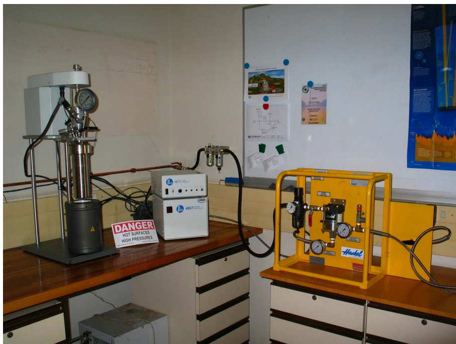
Figure 4.1: High temperature, high pressure Parr reactor connected to a liquid CO 2 pump
