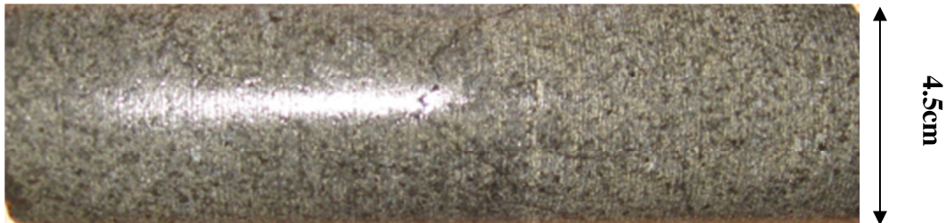
Figure 7: DO4 core sample with holocrystic texture
