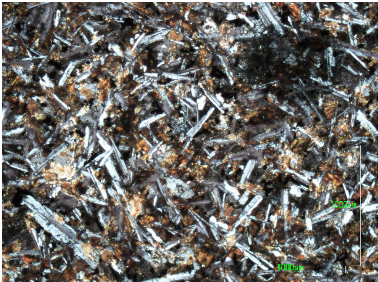
Figure 8: Photomicrograph of DO4 dolerite thin section under XPL.
