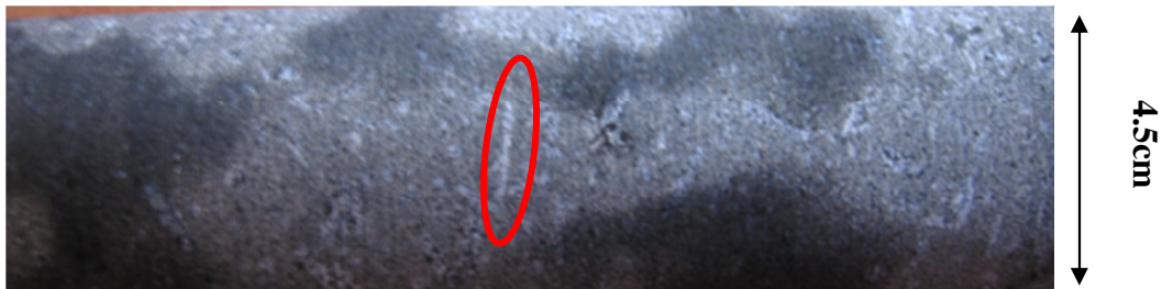
Figure 9: DO8 core sample with needle like phenocryst highlighted in red
