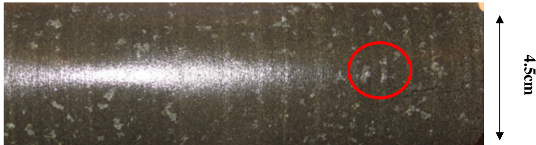
Figure 11: DO10 core sample with star shaped of nodular orientation of phenocrysts highlighted in red
