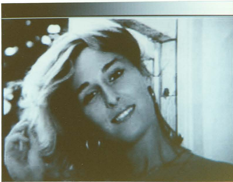
Figure 20 The image GIRL DCT coded to 1.0 bits/pel, using uniform quantisation with source encoding.
