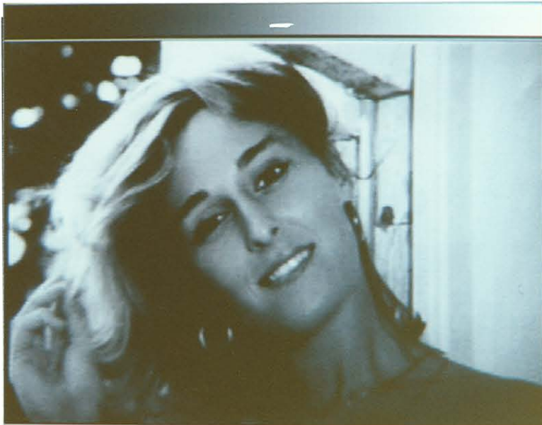
Figure 19 The image GIRL DCT coded to 2.0 bits/pel, using uniform quantisation with source encoding.
