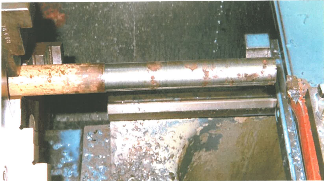
Figure 2.10. Corrosion products removed – deepest pits are visible.
