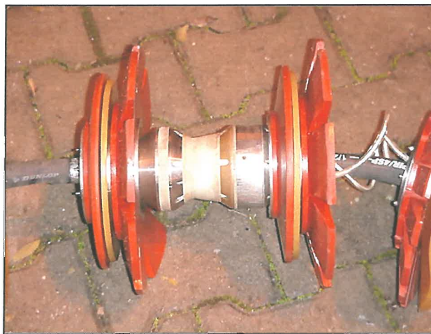
Figure 3.2. Intelligent “pig” used in ultrasonic thickness tests
