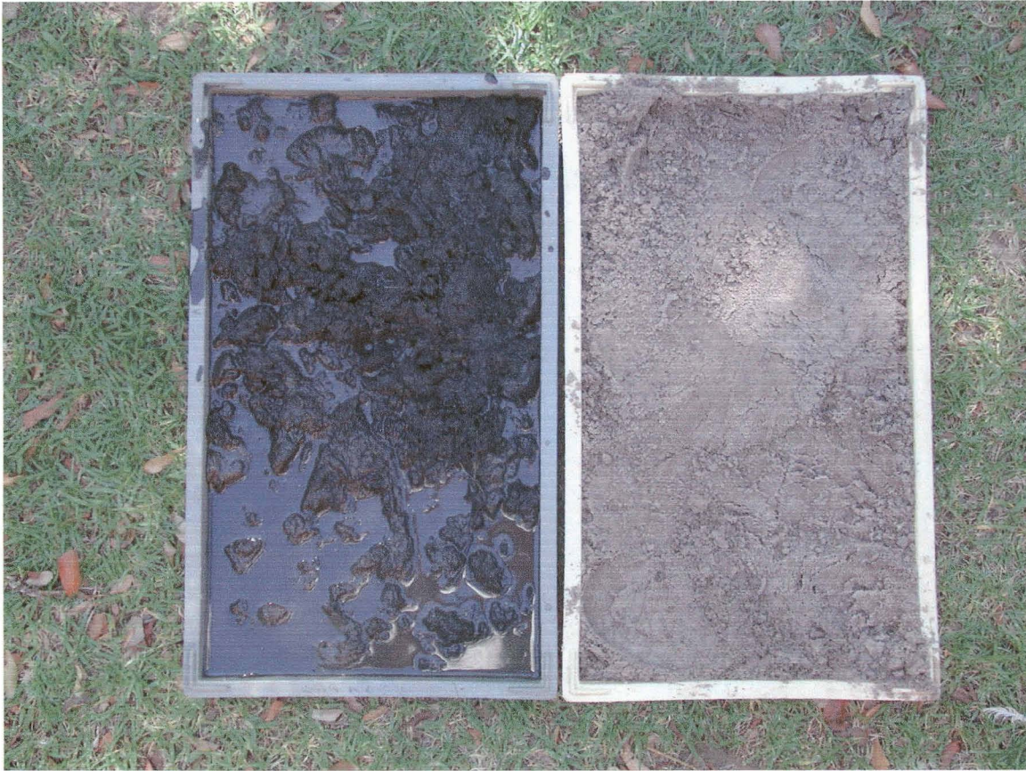
Plate 7.2: Samples of black material from the drainage ditch at the disposal site at Robertson 1 winery (left) and normal white soil from the disposal site (right)
