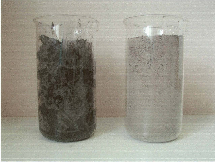
Plate 7.1: Samples of black soil from the water table at Robertson 1 winery (left) and white sand remaining after washing of a similar sample with water (right)
