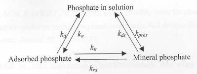
Where  $k_a$  = rate constant of adsorption.  $k_d$  = rate constant of desorption.  $k_{ds}$  = rate constant of dissolution.  $k_{pres}$  = rate constant of precipitation.  $k_{tr}$  = rate constant of transformation of adsorbed phosphate to mineral phosphate.  $k_{ra}$  = rate constant of re-adsorption of dissolved mineral phosphate.
