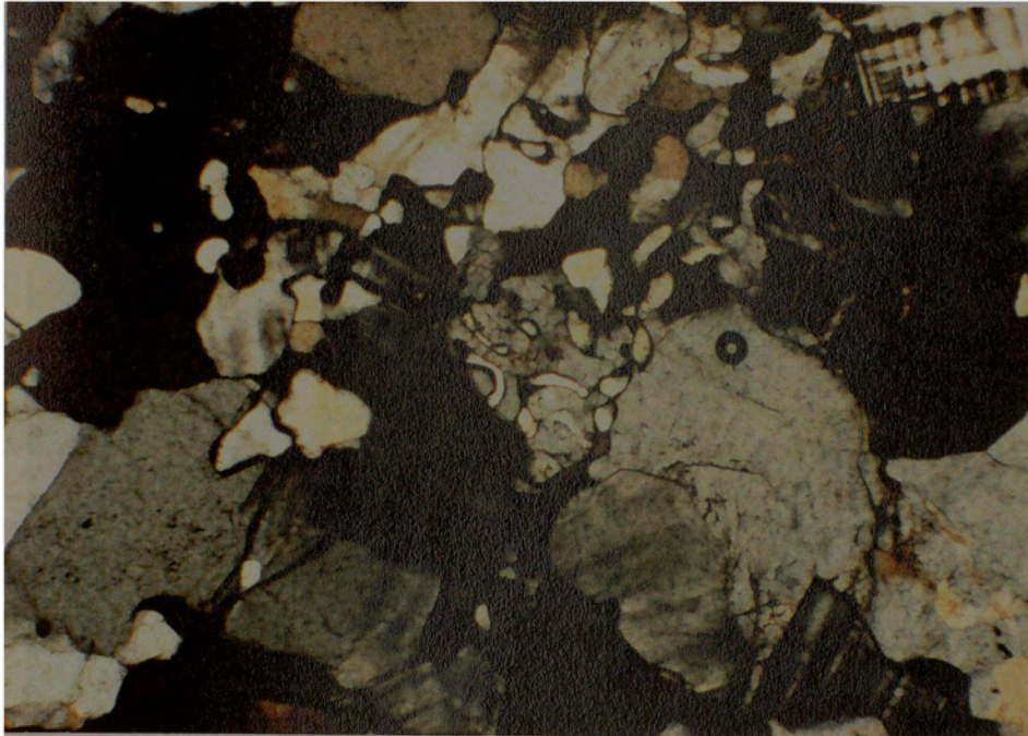
Figure 8.8: Myrmekitic intergrowths in the Nhansipfe Granitic Orthogneiss. Minerals in the photo are microcline (cross-hatch twinning), plagioclase (dark grey) and quartz (yellowish white). Crossed nicols, width of field 3 mm.
