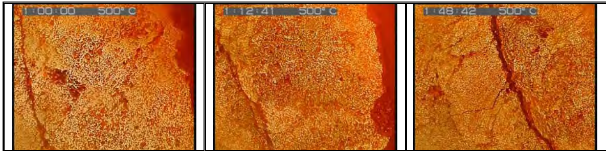
Figure 69: Optical microscope image during the high temperature microscope reduction test of Sample 16.
