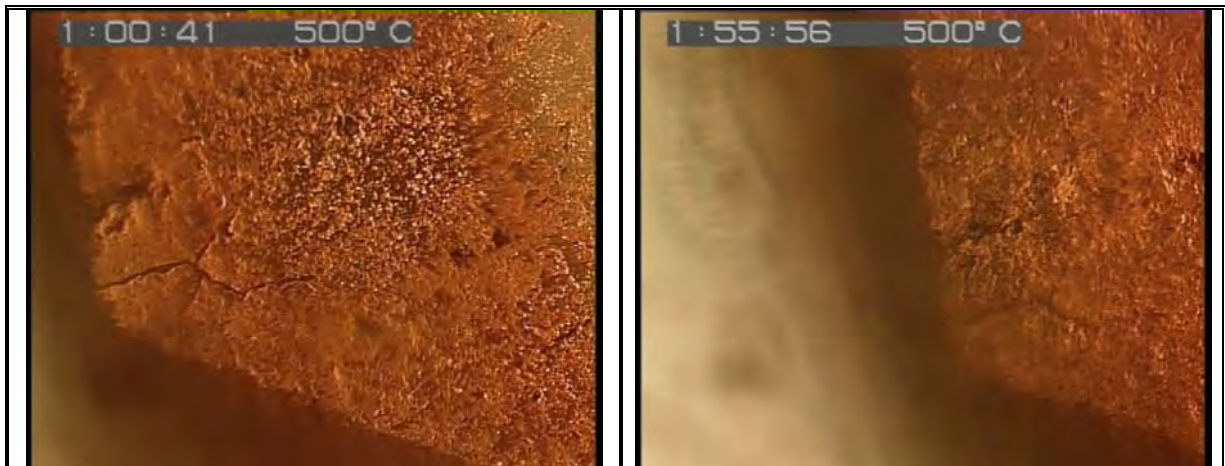
Figure 68: Optical microscope image during the high temperature microscope reduction test of Sample 15.
