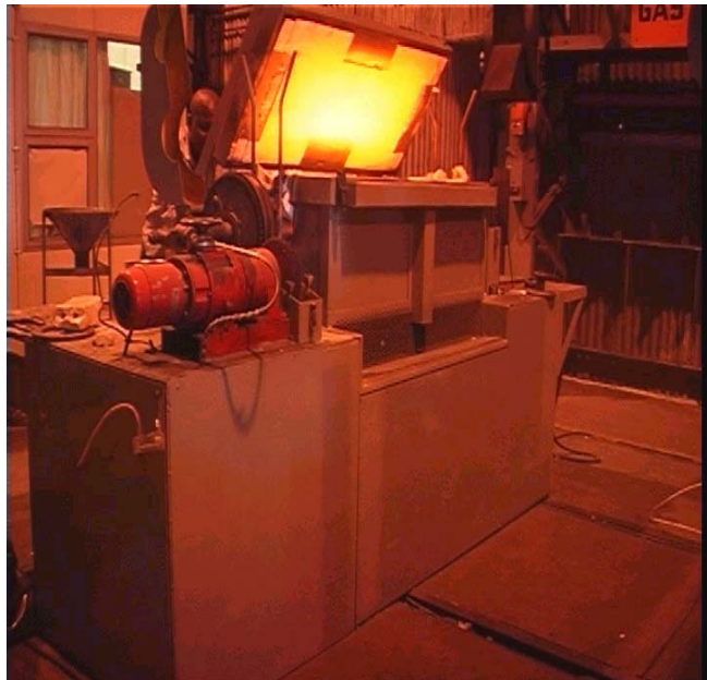
Figure 6: Photo of the COREX-Linder test apparatus at Kumba Iron Ore
