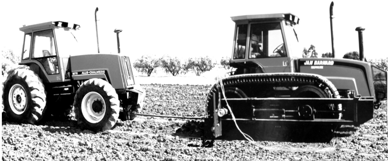
Figure 5.15. The tractors in series for the drawbar pull tests.
