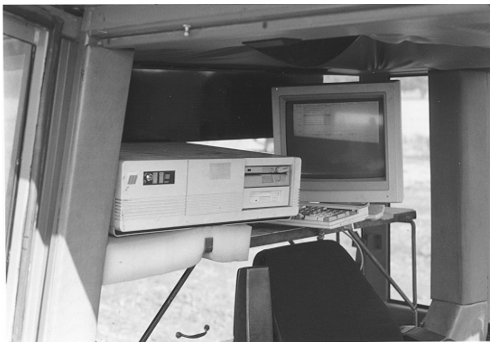
Figure 5.17. The computer system in the cab ready for data logging.
