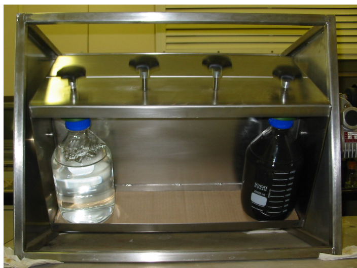
Figure 6.2 Experimental setup of the modified TCLP test
