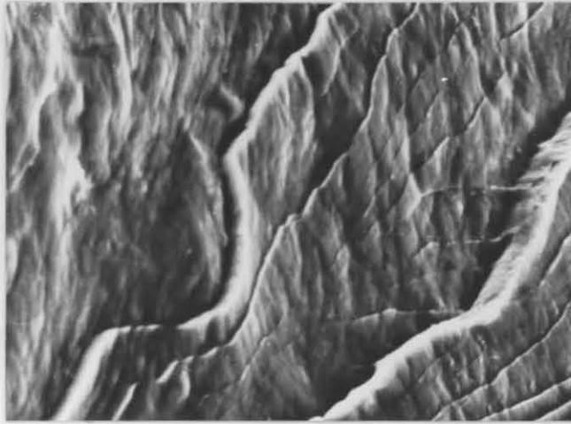
Figure 6.15: SEM micrograph of the split surface of a Charpy specimen showing a smooth undulating fracture surface (left) adjacent to a cleavage fracture (right) (1260X).
