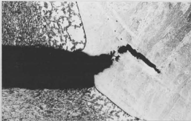
Figure 5.21: Stable crack extension in the 309L weld metal of a through-thickness crack in a fractured FLNFT specimen (35X).
