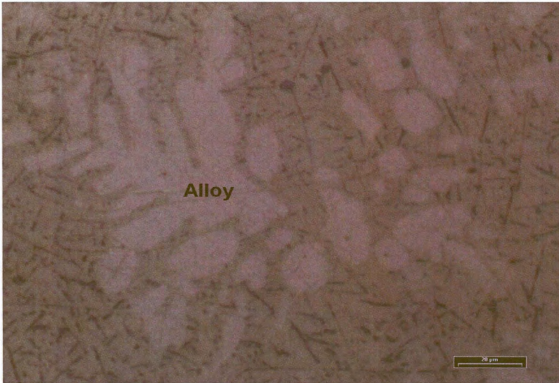
Photograph 5.3: Melt with skeletal alloy growths (experiment 10e1).
