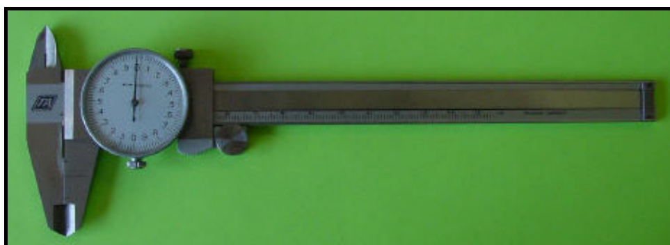
Figure 28: Dial caliper used for measurement of the overbite
