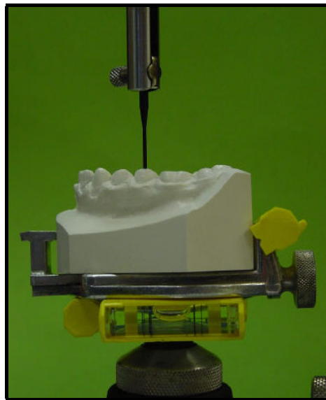
Figure 9: The analysing rod of the dental surveyor was used to standardize the vertical height of the dental casts
