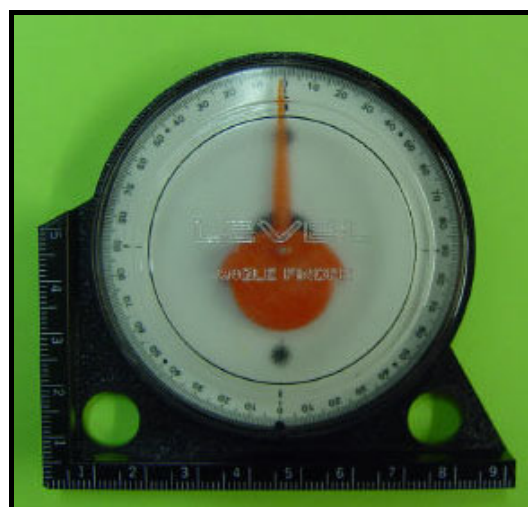
Figure 14: An angle finder with millimetre ruler used for calibration of photographs
