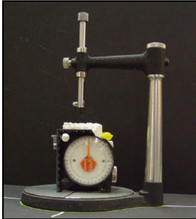
Figure 17: Setup of the dental cast and surveyor
