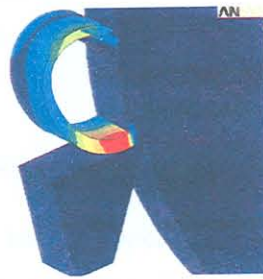
Figure 2.16: Explicit dynamic FEM model of the machining process [69]
