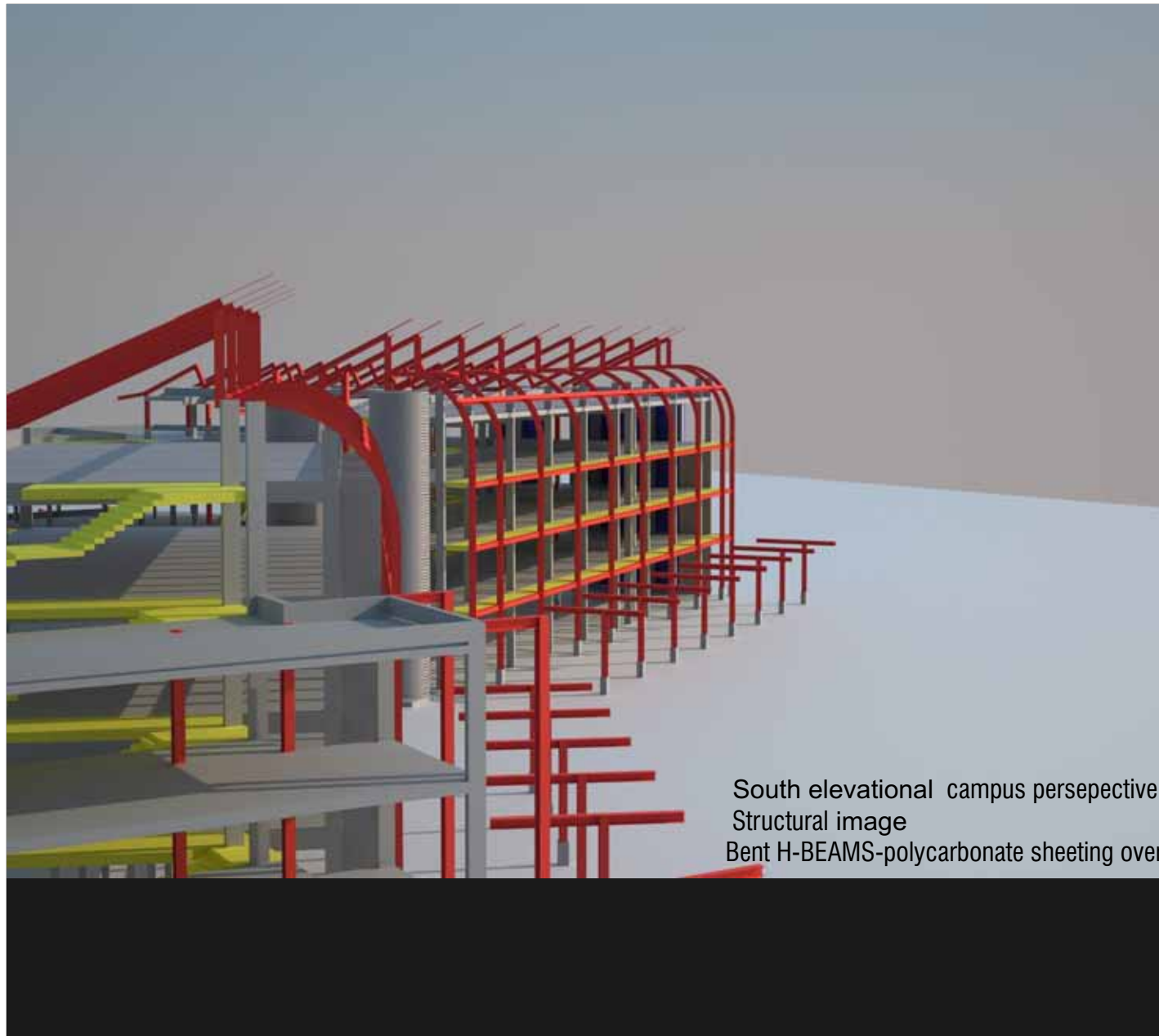
Public square, concrete base, Steel columns
