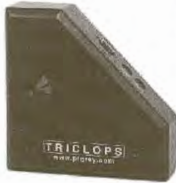
Figure 2.2. An example of a Stereo camera that is used in immersive environment (Triclops stereo camera, developed by Point Grey Research Inc.) [46].
