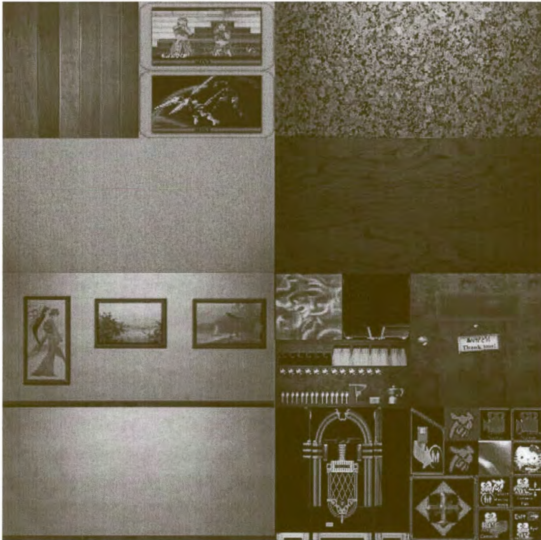
Figure 5.9 A single texture containing all the textures of the virtual pub environment and the virtual objects.
