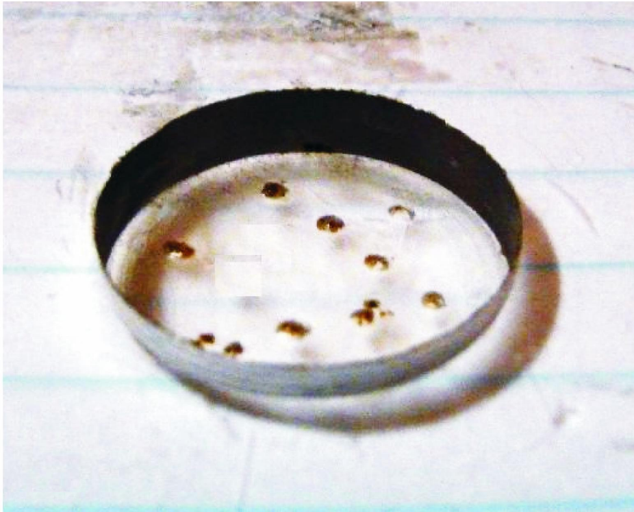
Figure 4.2: This figure shows the microphone-diameter blind hole. The smaller holes at the bottom of the larger hole were drilled for method 5, but were not present in method 3.
