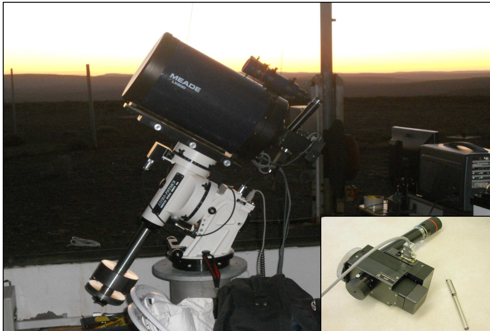
Figure A4.2. The SALT MASS-DIMM in operation at the SAAO site in Sutherland with the MASS-DIMM instrument attached at the exit pupil displayed in insert bottom right.
