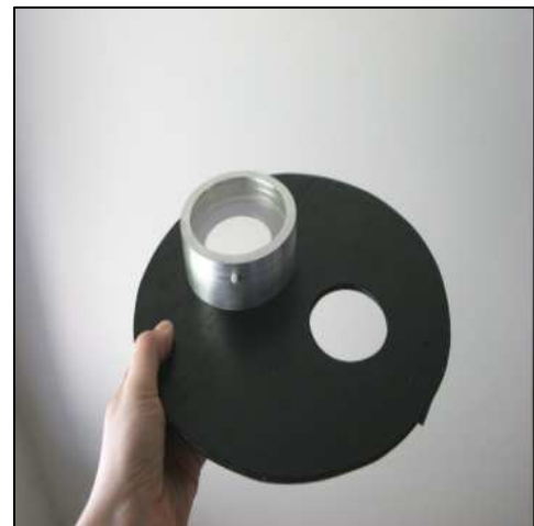
Figure A4.1. DIMM mask with wedge prism (source: Andrei Tokovinin).
