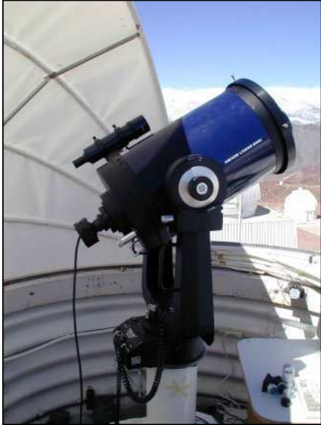
Figure 4.7. The Cerro Tololo Inter-American Observatory (CTIO) Robo-DIMM in Chile with motorised canvas clamshell enclosure (source: CTIO).
