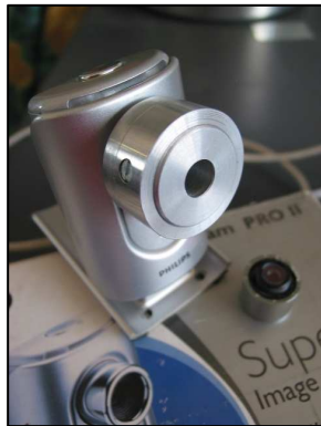
Figure 4.4. The Philips ToUcam Pro II PCVC840K webcam with lens removed and replaced by MOGG adapter.
