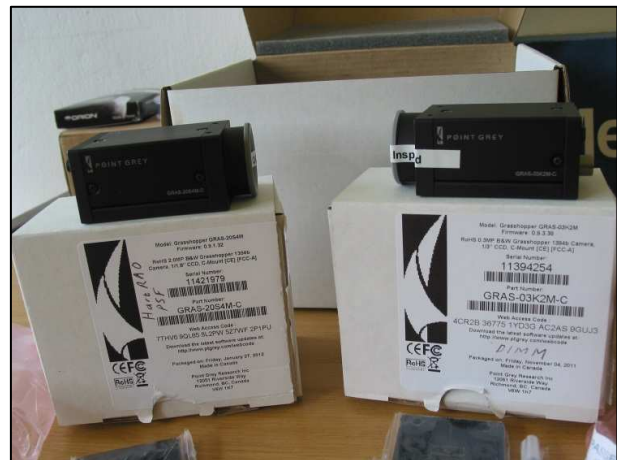
Figure 4.3. The Point Grey Grasshopper GRAS-03K2M (for DIMM measurements) and GRAS-20S4M (for PSF seeing monitor measurements) CCD cameras.
