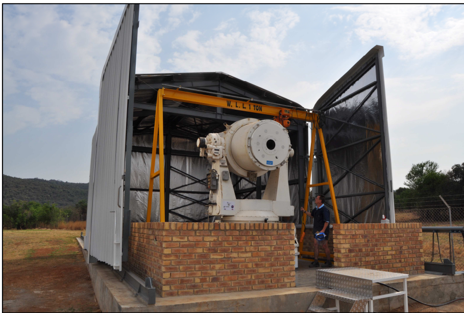
Figure 1.4. The OCA 1-m aperture Cassegrain telescope mount and tube at HartRAO.
