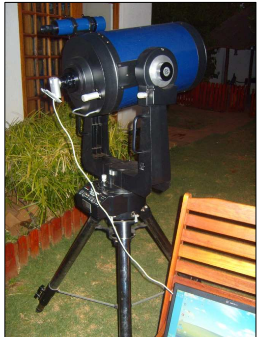
Figure 4.5. Test setup for double star observation – 10" Meade LX200 SCT, ToUcam webcam and laptop.
