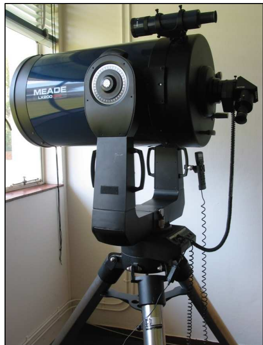
Figure 4.2. Recently acquired second-hand 14" Meade LX200 GPS SCT with alt-az fork-arm mount and field tripod.
