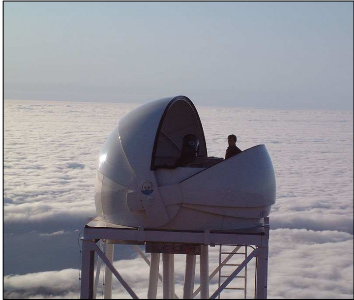
Figure 4.8. The Isaac Newton Group of Telescopes (ING) – Instituto de Astrofísica de Canarias (IAC) RoboDIMM with Astro Haven fibreglass clamshell at the Observatorio del Roque de los Muchachos (ORM) La Palma, Canary Islands (source: Javier Méndez, ING).
