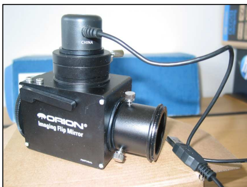
Figure 4.6. The Orion StarShoot USB Live View Value Kit with imaging flip mirror and StarShoot USB eyepiece.
