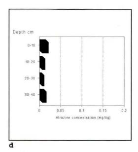
**Figure 7** Leaching pattern of atrazine as depicted by estimated residual atrazine in different soil layers: (a) 30 days after treatment (d.a.t.); (b) 60 d.a.t.; (c) 90 d.a.t.; (d) 120 d.a.t.
