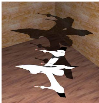
Figure 3.18 Rendering a shadow by means of a shadow map (via one light source and three-dimensional mesh) – accurately cropped and skewed to fit the surrounding area.
