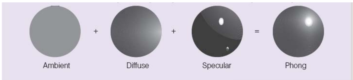
Figure C.15 Combining the lighting terms, producing a Phong reflection
