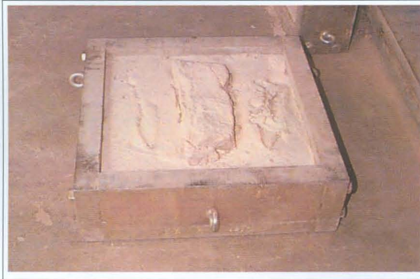
Figure 3.6 Bottom half of shear box assembly with test specimen
