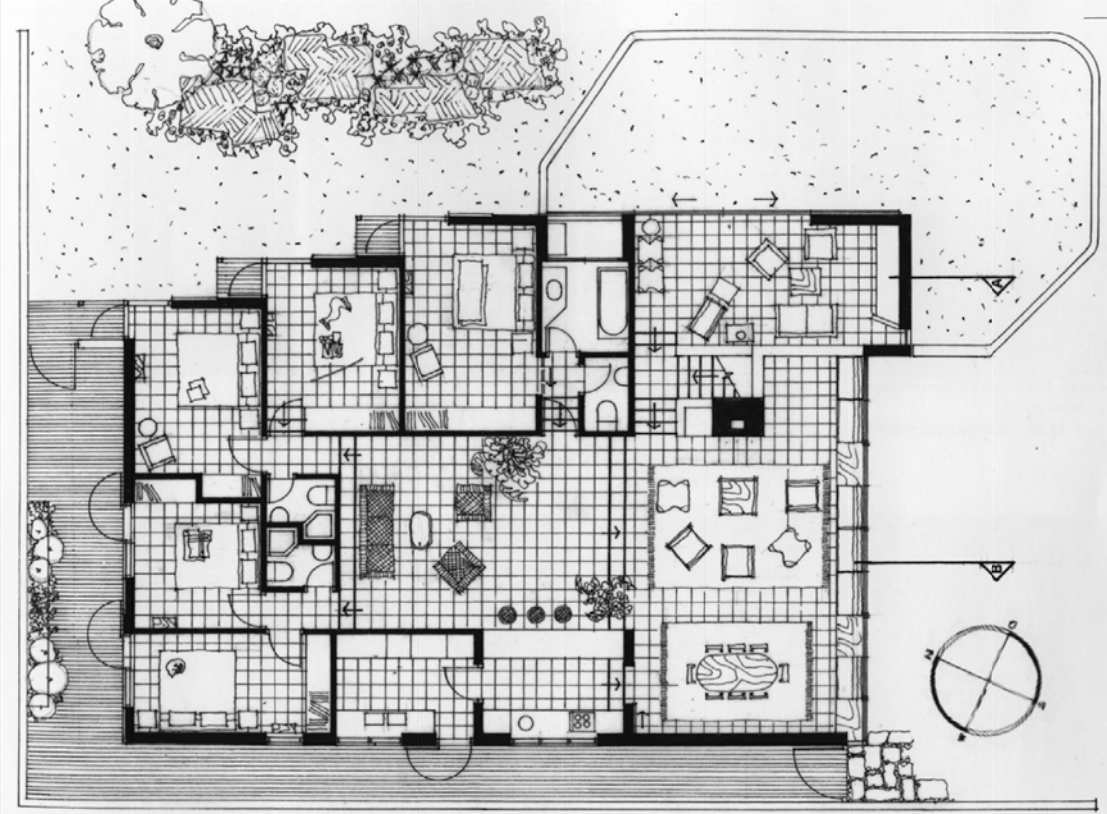
Figure 7.19. Top: Boundary walls merge building with landscape at House Swanepoel in Hermanus (1991) (Author, 2008). Bottom: Plan of House Swanepoel Hermanus showing tight service and generous living spaces (Fagan, 2005a:103).
