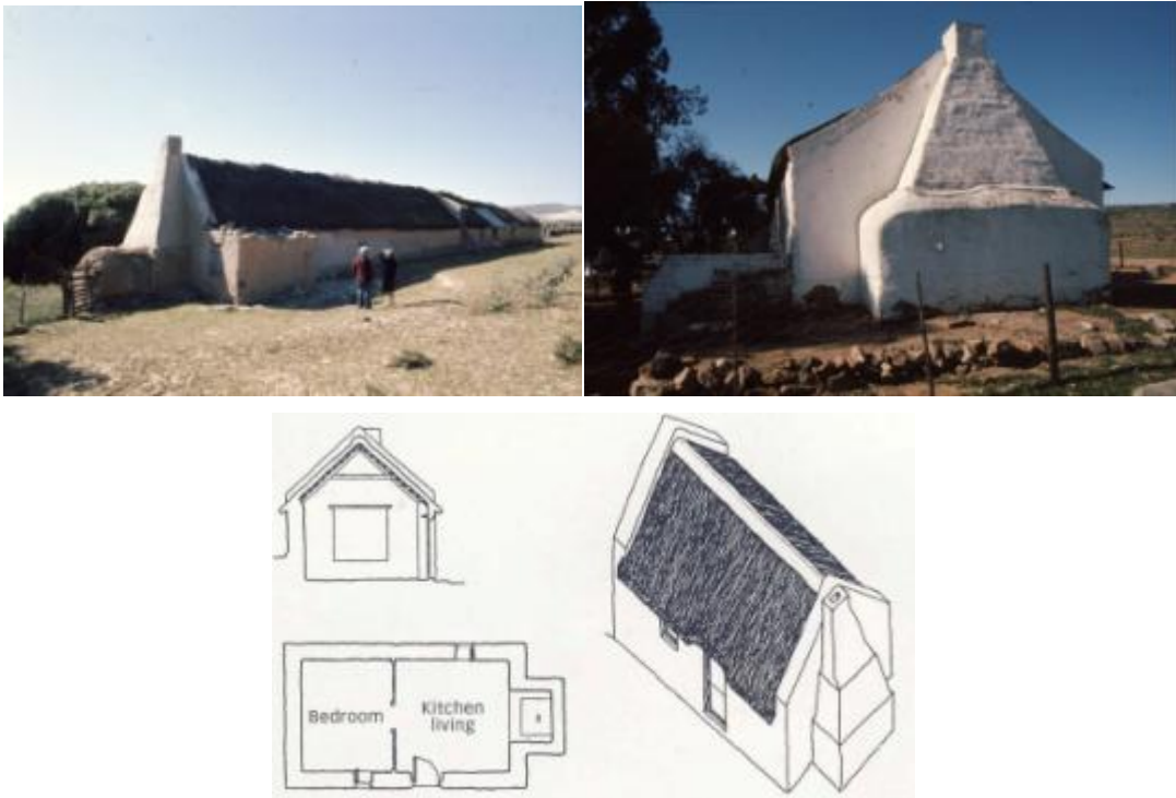
Figure 3.2. Top: Vernacular houses in Velorenvlei photographed in June 1972 (Fagan slide archive EM, undated). Bottom: Plan, section and axonometric of typical 19th-century vernacular dwelling in Struisbaai, Southern Cape (Japha, 1997:2159).
