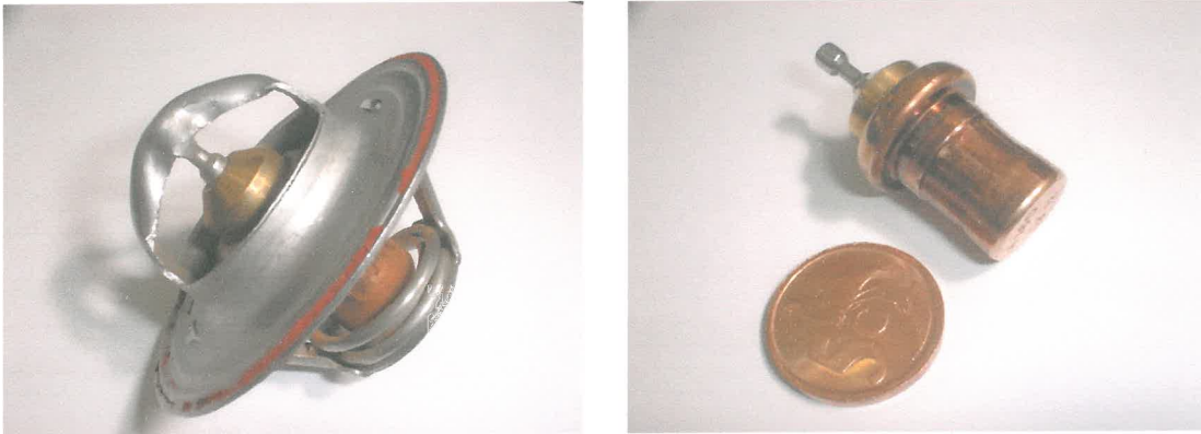
Figure 3.22 Thermostat and wax actuator
