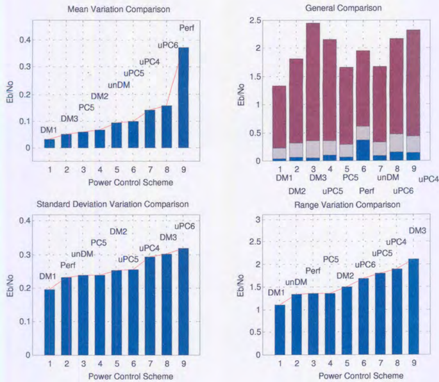
FIGURE 5.8: Mean variation, standard deviation and range comparisons for different FPC pdf algorithms are depicted in this figure with an AWGN channel, R_x=2 , i=1 , RAKE fingers=3, N=32 and matched-filtered W-CDMA system.
