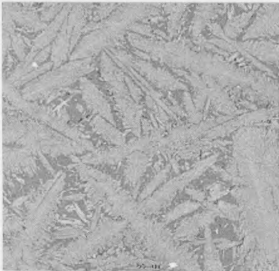
Figure 4.19: SEM backscattered image of the mould flux of the ferritic steel with 10% Ti_2O_3
