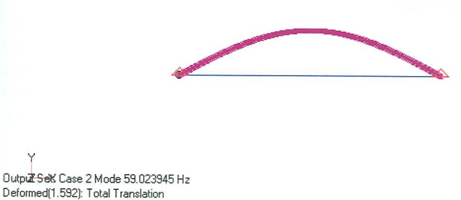
Figure 2.8 a) Mode shape of tube with length 0.8635 m with pinned supports
